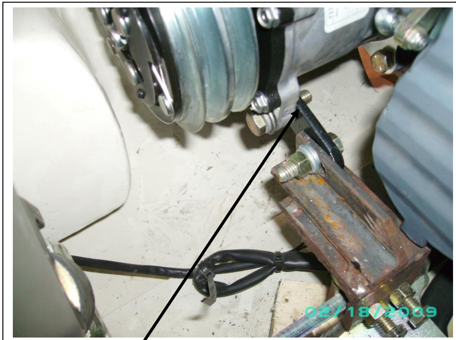
Inside lower ear supported by bracket which clamps as shown.
