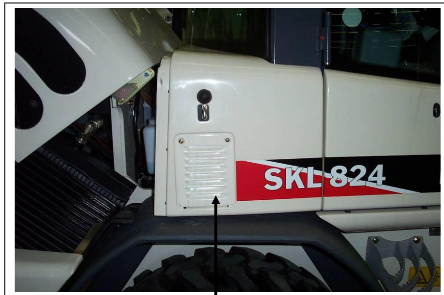
Air intake panel back in place.
